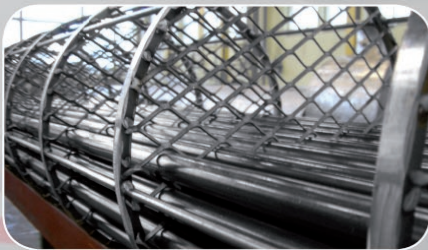
An example of an 18 metre, Compact EMbaffle® Gas/Gas heat exchanger under fabrication
